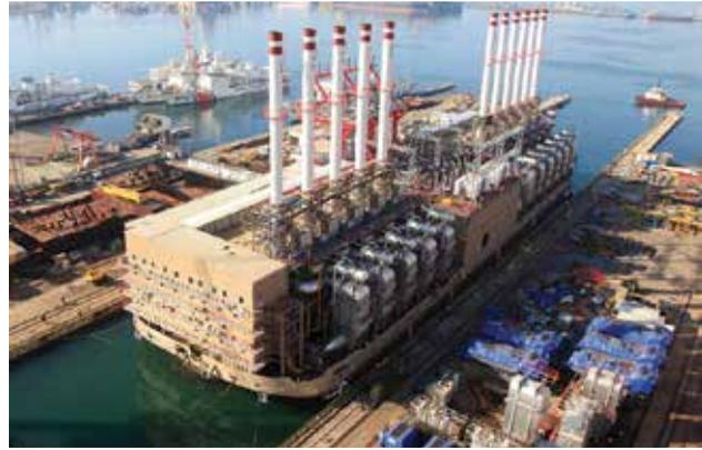
combustion engines). In addition to having the highest efficiencies, Powerships can be transported to different coastal locations based on the utility’s requirements. Powerships’ large capacities enable them to supply the base-load power of a whole country. All accommodation facilities are also located on-board.
